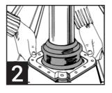
Slide down the pipe using water as a lubricant.
