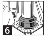
Fasten using self drilling washered screws or sealed rivets.
