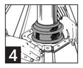
Press base to roof profile by hand.
